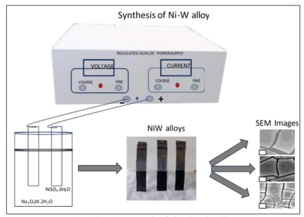
Fig. 1. Schematic Representation of Ni-W Electrodeposition.
