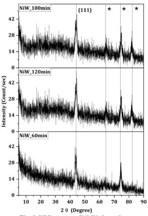
Fig. 2. XRD pattern of Ni-W electrodes.
