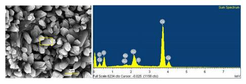
Fig. 13. SEM image and EDAX elemental analysis of hexagonal calcite crystals.
