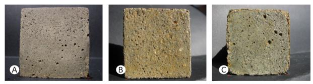
Fig. 3. PC5 mortar specimens exposed to sodium sulfate solution after A: 70 days, B: 140 days, and C: 280 days.
