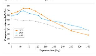
**Fig. 5.** Compressive strength of specimens subjected to sodium sulfate solution.
