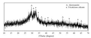
Fig. 1. X-ray diffraction pattern of BFS
