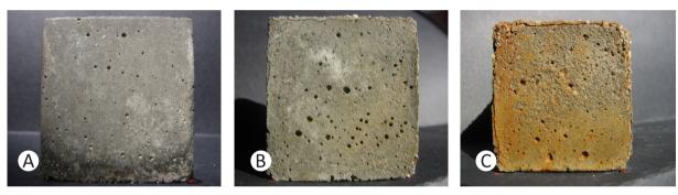
Fig. 2. PC2 mortar specimens exposed to sodium sulfate solution after A: 70 days, B: 140 days, and C: 280 days.
