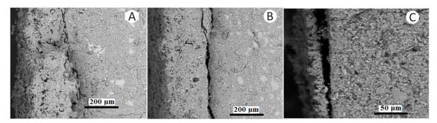
**Fig. 10.** SEM images (BSE mode) from cross sections of regions close to the exposed surfaces of the A) PC2, B) PC5, and C) AAS paste specimens.
