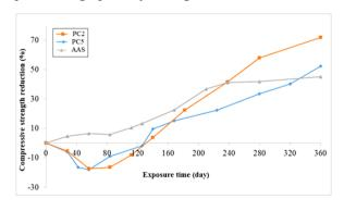
**Fig. 6.** Compressive strength reduction of specimens subjected to sodium sulfate solution.
