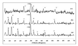
Fig. 9. XRD patterns of paste specimens exposed to 5% sodium sulfate solution: (a) PC2, (b) PC5, and (c) AAS. (E=Ettringite, G=Gypsum, C=Calcite, CSH= calcium silicate hydrate, A=Akermanite).
