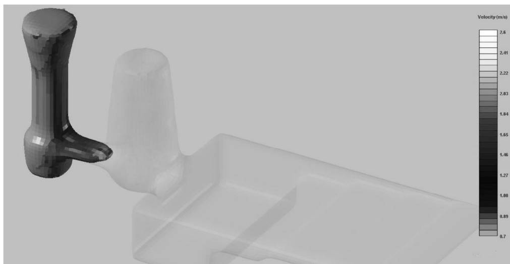
Fig. 10. The melt flow velocity in the runner of the specimen cast without any filter. (1840 mm/s)
