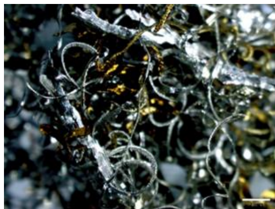
Fig. 1. AA 7075 swarf produced from the machining process
