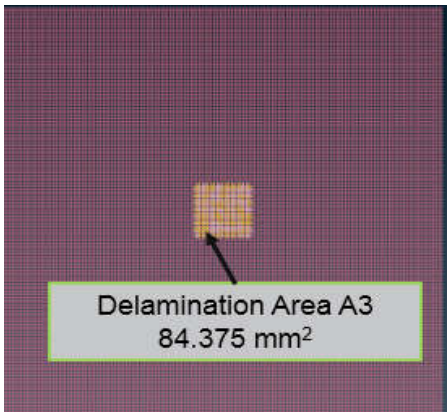
Fig. 3. Top view of delamination incorporated.
